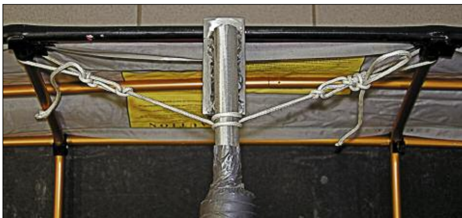
New yoke with strings attached to prevent forward and aft movement
