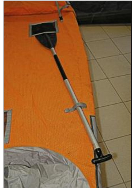
The original spare paddle apparatus on the right side. Paddle grip points towards the stern
