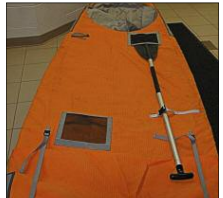
The modified spare paddle apparatus on the left side. Paddle grip points towards the bow
