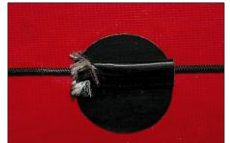
Wear on the spray-deck attachment patches from bashing through ice-pans
