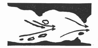
Standing waves pile up at the base of a drop: the first wave is the largest and steepest..second wave large, but smooth and regular. Split the waves dead-on (bow first). The faster your speed, the more your bow will tend to bury itself in the wave and cause water to break over the gunwhales. Hard back-paddling will minimize speed and give your canoe time to lift over the wave.
